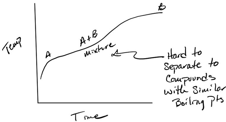
③ Two Component mixture A + C w/ different Boiling Points
